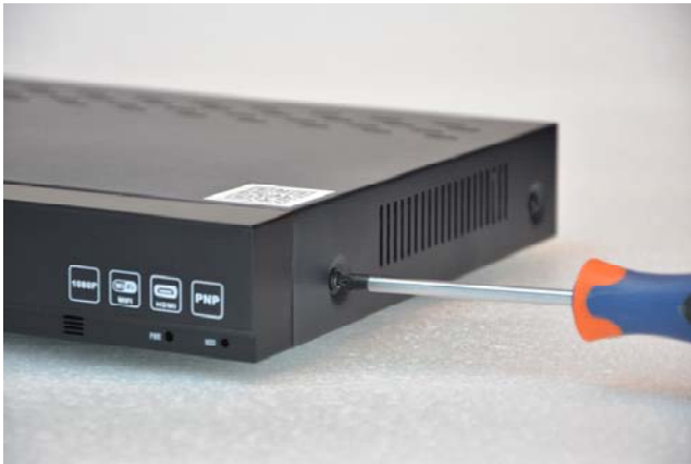
Remove the cover by unscrewing the 5 screws: 2 on each side and one rear
