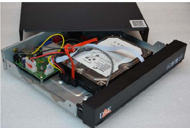
Secure the hard drive with the 4 screws provided that you screw from under the base. Then close the cover.
